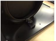
Install the Mac pro as shown. Either bay is available. Use the left bay If you plan on using the SanLink adaptor. The tabs that are at the front of the nesting opening will insert into the cooling vents on the bottom of the Mac Pro® (shown right). It may be necessary
